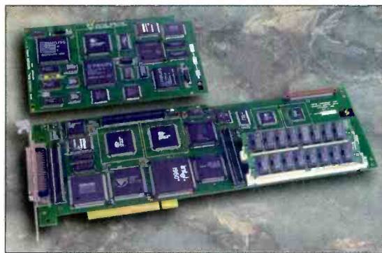
The analog daughtercard and the main board of the Multistream Xpress.
